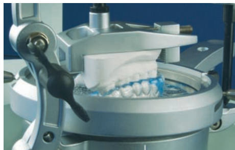
8. The upper or lower model is placed in the Erkoform-3d to thermoform the splint and create the flat bite table.
